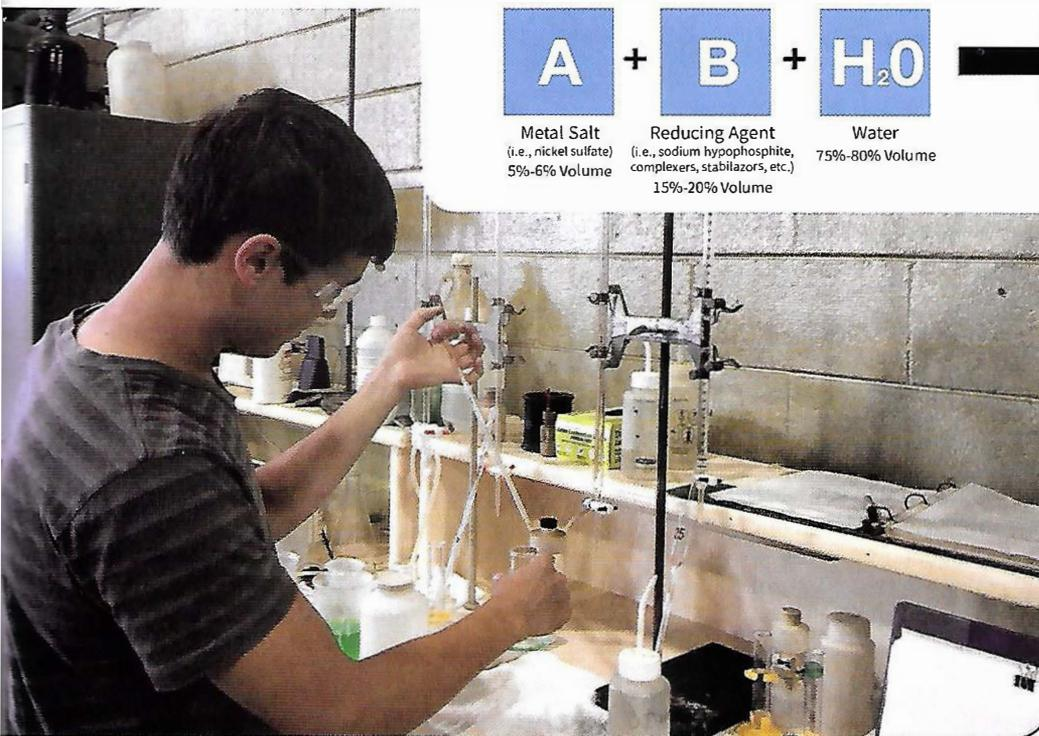
Surface Technology has pushed the One-Plate concept as a simpler way to manage EN baths, with less chance of human error.
